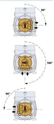
When rotating the pump body it is also necessary to rotate the pump body back-plate
